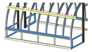
Figure 33. Final location of purlin ready for attachment to ribs.
