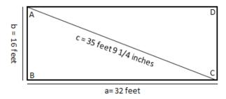
Figure 5. Perimeter points used to establish a square structure.
