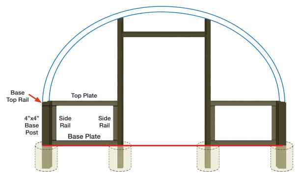
Figure 28. End wall assembly.
