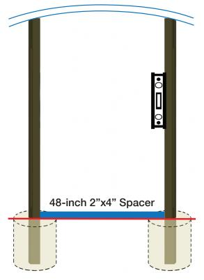
**Figure 25.** Placement of second post, using a 48-inch spacer.
