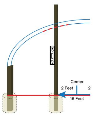
Figure 23. Placement of first post for door frame.
