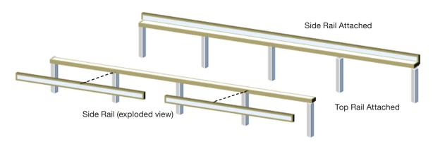
Figure 10. Top rail assembly, including temporary guide rail attachment.
