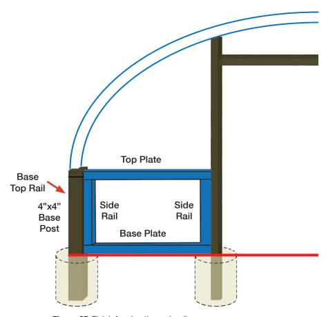
Figure 27. Finish framing the end walls.
