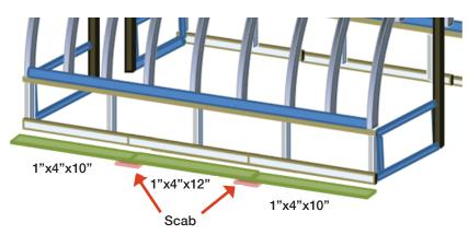
Figure 31. Purlin configuration with scab locations to avoid ribs.
